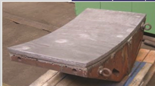
Hydrostatic pad
