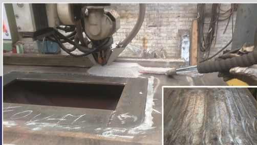
Strip cladding process
